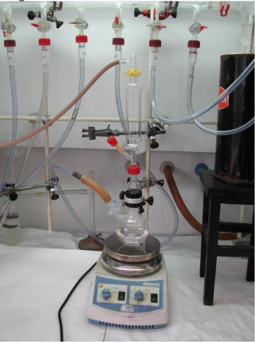
• The top of the funnel uses a "duck head" adapter to connect to the gas line using flexible tubing (preferably Tygon). For aerobically stable reagents and
